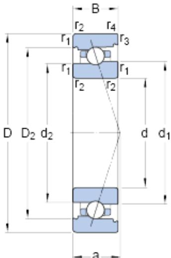
7017 ACB/P4A Bearing 2D drawings and 3D CAD models
