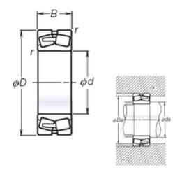
45 mm x 100 mm x 36 mm NSK 22309L12CAM spherical roller bearings
